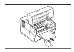
**NOTE:** If the jammed paper appears to be pinched by rollers, pull it along the normal running direction of the paper.
